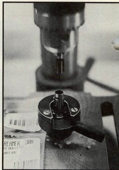
Reaming out the neck of the newly formed case in a drill press.
