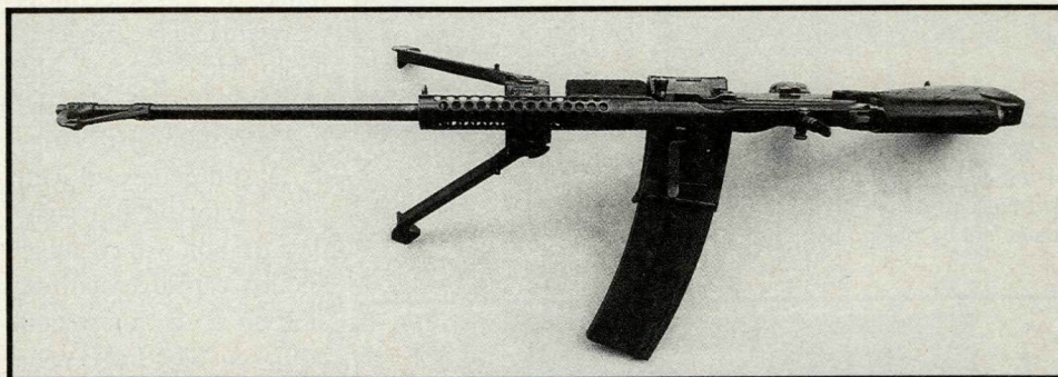
A top view of the Johnson Model 1941 shows the side-mounted, single-column magazine, which was too long and threw off the balance of the weapon.
